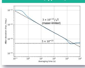
Tiqker is 50 times more stable at 10 second averaging time and 1000 times faster to 10 <sup>-13</sup> frequency stability as compared with standard cesium beam references
