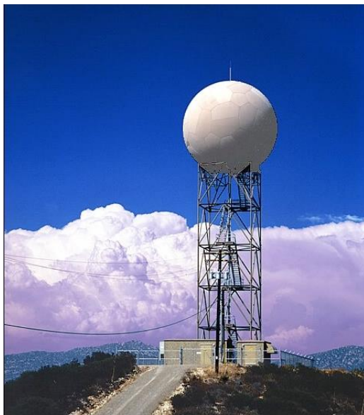
Figure 1.1: A Doppler radar for the forecast (measure the speed of the rain and the hail) and the severe storm research in Kansas City, US [1].
